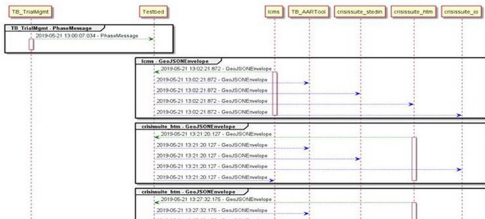
Figure 16. AAR sequence diagram, showing the interaction between filtered systems.
